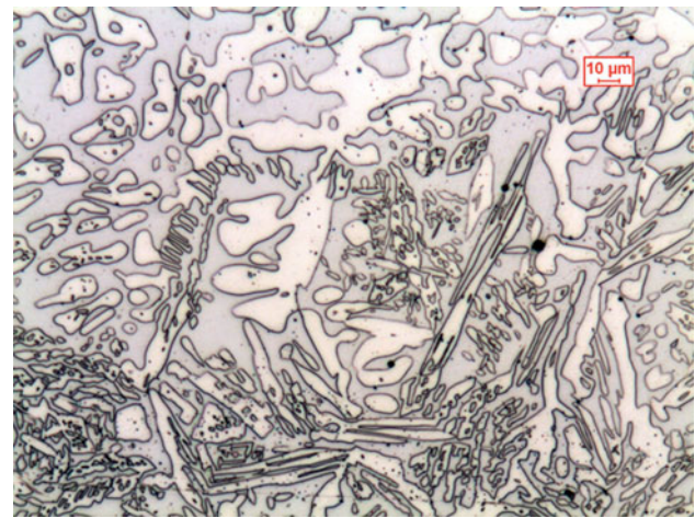
Fig. 8 HAZ micrograph of the solution-treated specimen (1100 °C) showing the growth of austenite particles in place of precipitates
